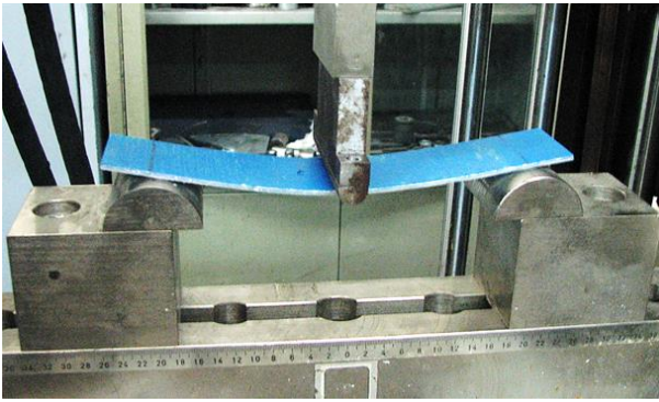
Figure 1. Test setup for three-point-bending test of FS1 specimen.
