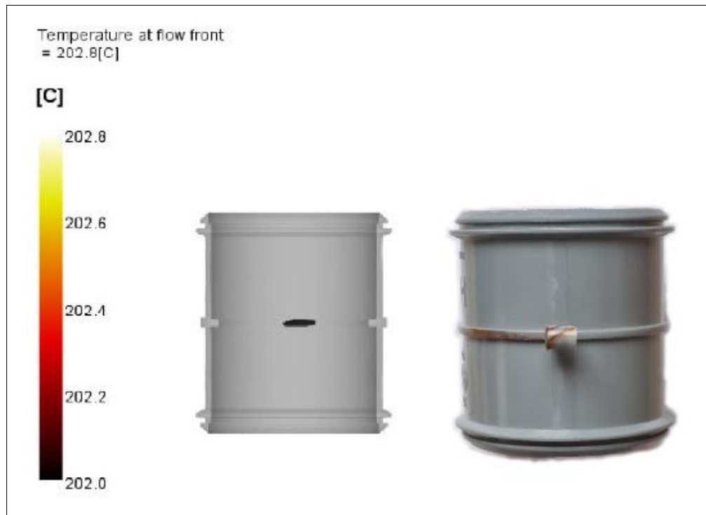
Fig. 3: Burn mark defect in Experiment 2
