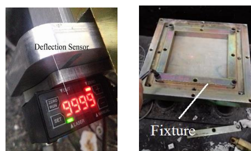
Figure 3. Deflection sensor and fixture
