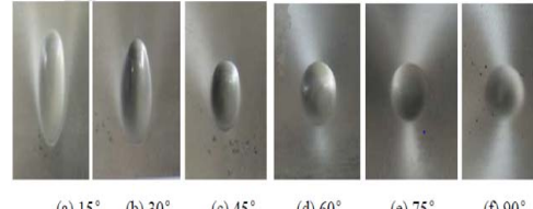
Figure 2. Macrograph of corrosion scars caused by different angles of contact of solid particles
