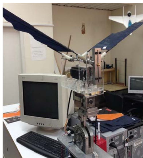
Fig. 2. The experimental test setup constituted flapping wing and load-cell
