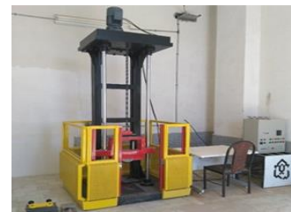
Fig. 4. Drop hammer test machine 7500 J
