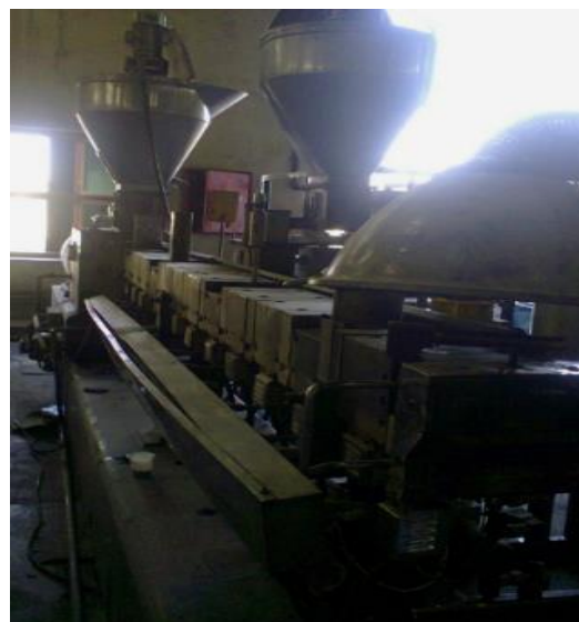
Fig. 1. The used twin screw extruder
