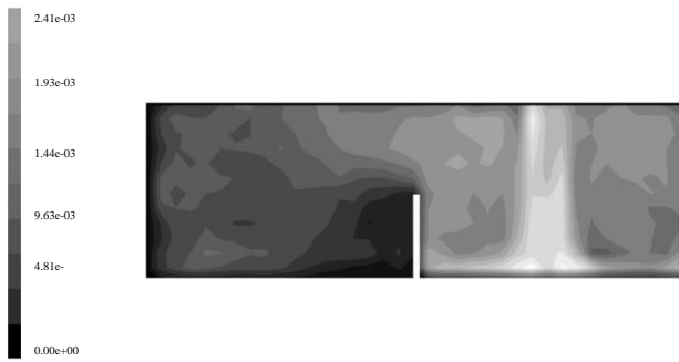
Fig. 4. 1 \mu m particle concentration contours at the mid-plane of the room at t=130 s.
