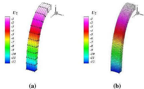
Fig. 2. Deformed shape and displacement contours in z direction for the IGA (left) and FEM (right)
