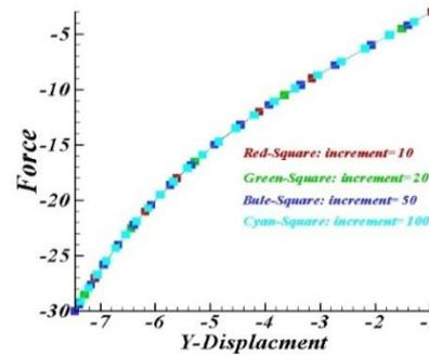
Fig. 7. Vertical displacement of the loaded point with different load increments
