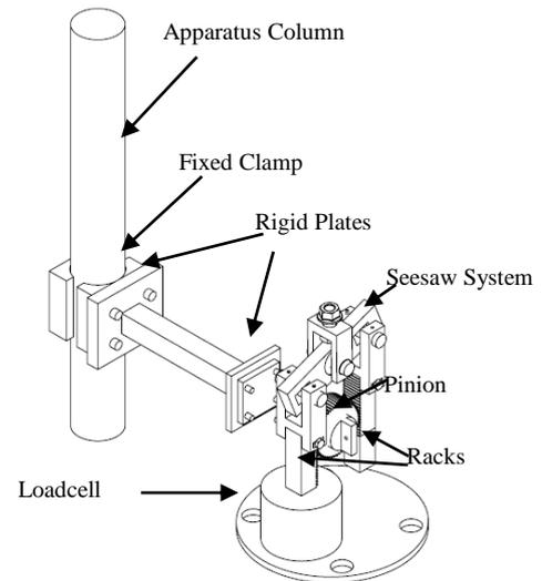
Fig. 1. Pure torsional loading fixture
