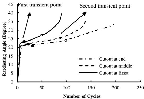
Fig. 3. Ratcheting angle vs. number of cycles for cubic shell with circular cutout in different positions
