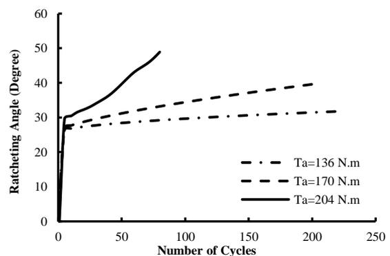
Fig. 2. Ratcheting angle vs. number of cycles for cubic shell with circular cutout in different positions
