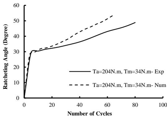
Fig. 4. Comparison of experimental results with finite element method of ratcheting angle for cubic shell under torsional loading with amplitude of 204N.m and mean magnitude of 34N.m
