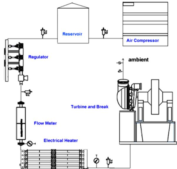
Fig. 1. Schematic diagram of turbine test rig
