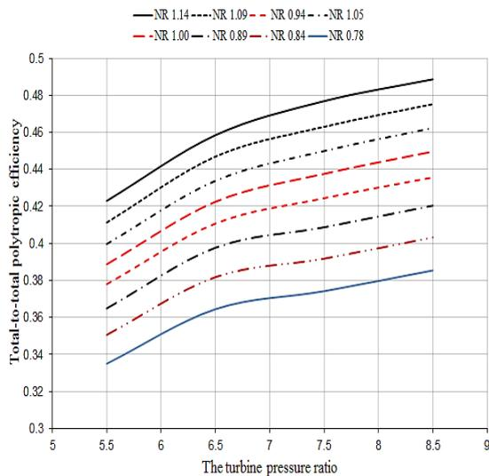
Fig. 4: The turbine characteristic curve in different rotational speeds
