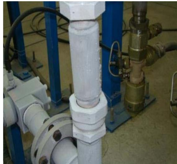
Fig. 2. Ice formed on the pipe after pressure regulation
