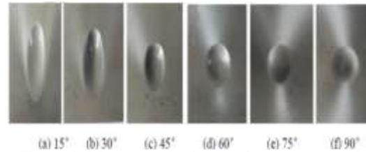
Figure 2. Macrograph of corrosion scars caused by different angles of contact of solid particles
