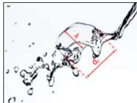
Figure 3. Measurements on a bag
