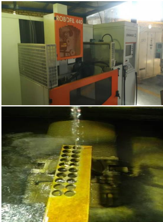
Figure 2. Five-axis wirecut machine and fixing the workpiece on it
