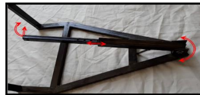
Fig. 2. Support base and movable arm to adjust the angle in three dimensions
