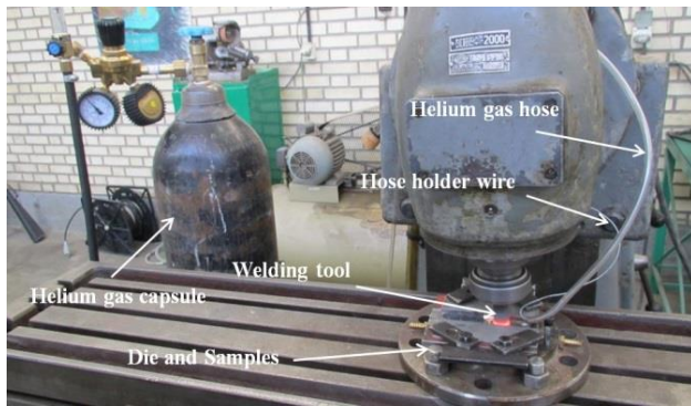
Figure 1: Copper plates and die and its accessories
