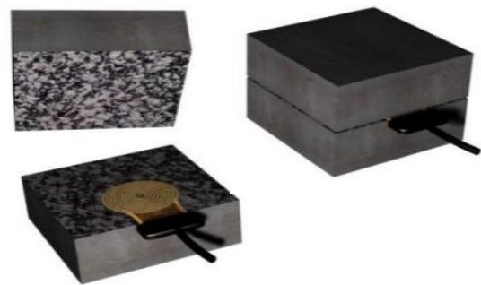
Fig. 7. Transient plane source method [39]
