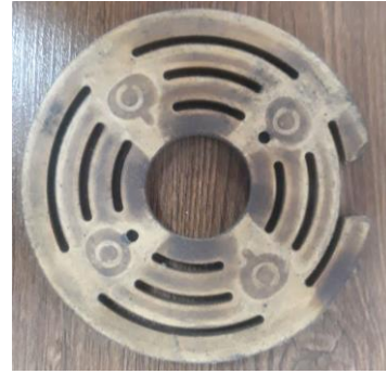
Fig. 7. Fault on the Valve Disc
