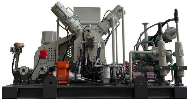
Fig. 1. The reciprocating compressor
