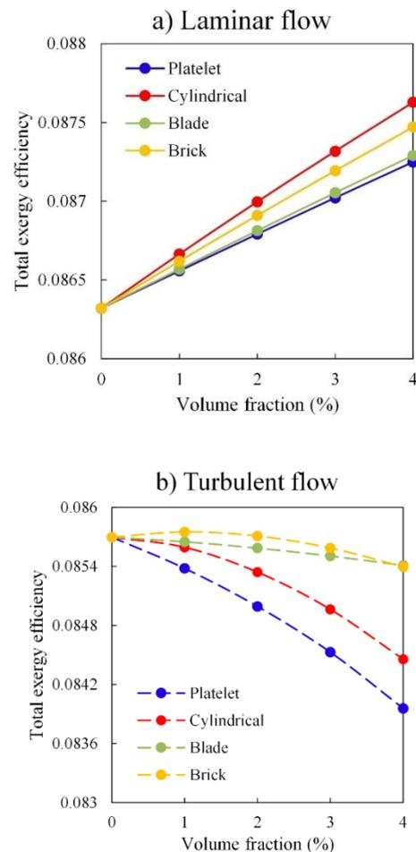
Fig.2. Variation of total exergy efficiency with volume fraction for different nanoparticle shapes in laminar and turbulent regimes.
