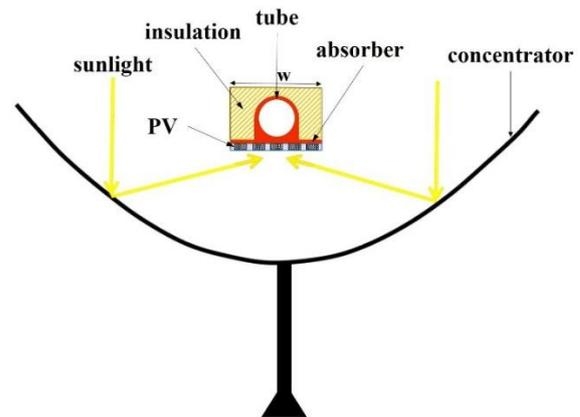
Fig. 1. Concentrating photovoltaic/thermal system.
