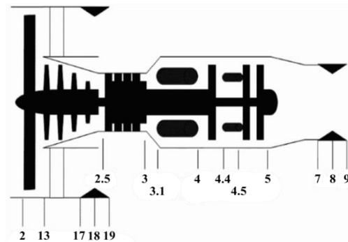
Fig. 2. Different stations turbofan engine with a secondary combustion chamber.
