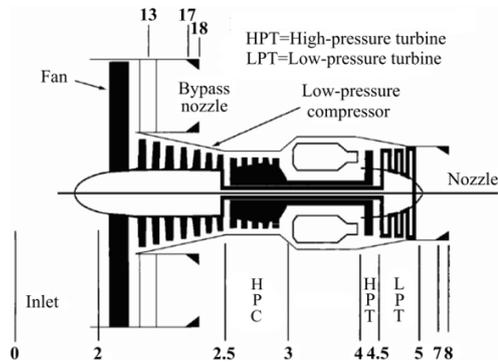
Fig. 1. Different stations turbofan engines without secondary combustion chamber.
